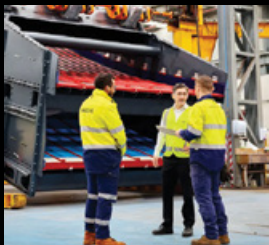
Stationary vibrating screens
